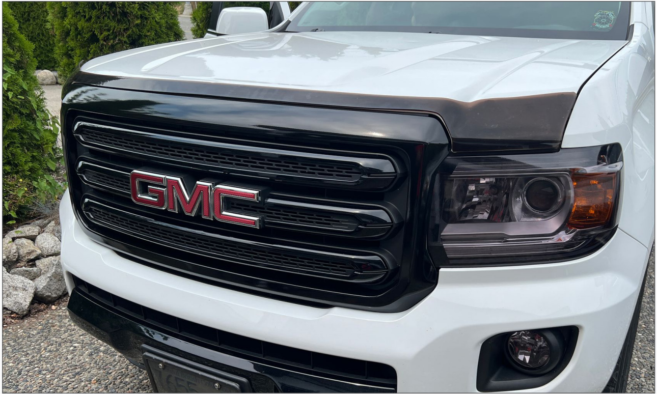
AFTER: Vinyl Wrapped Grill Frame (Black), Wrapped Headlight/Fog Light (Tinted Clear)
