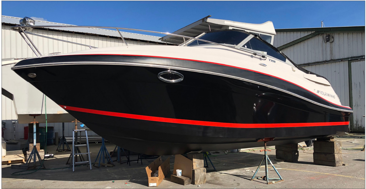
Boat Wrap - Black on Hull, above water line
